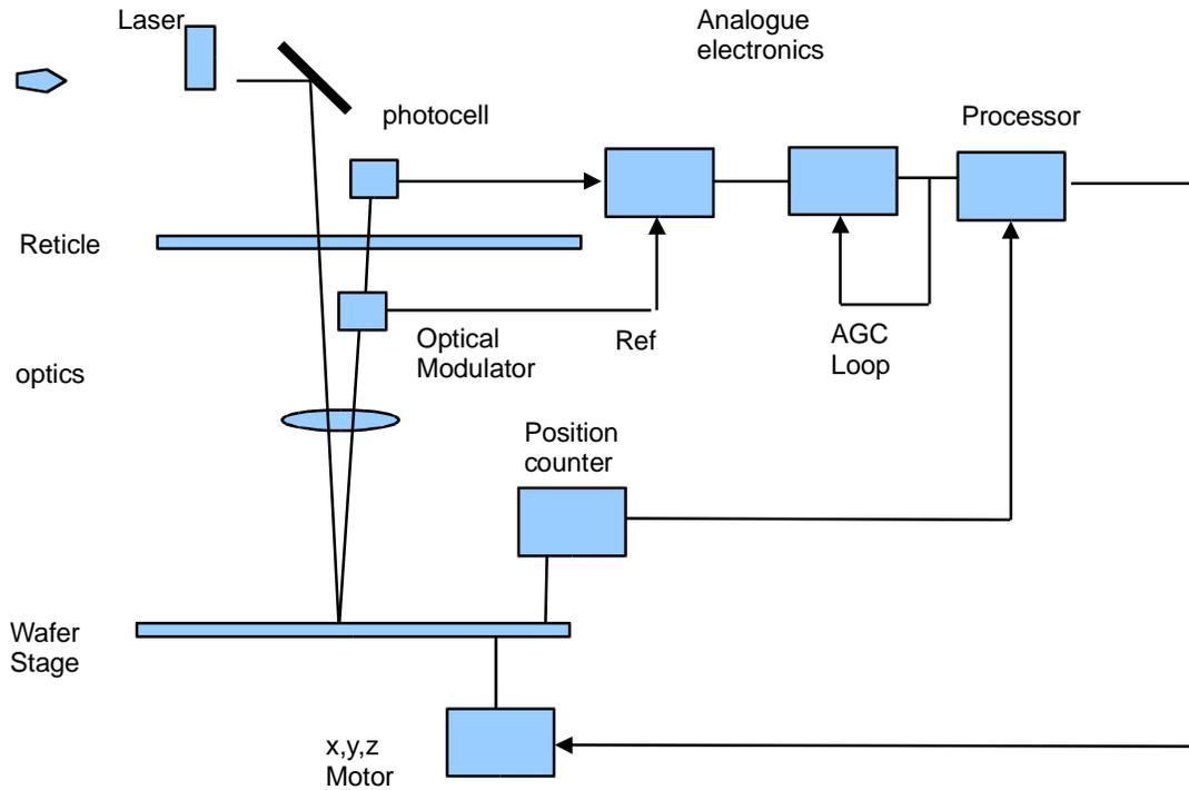
**Fig 3: Alignment System with AGC and Synchronous Detection**
