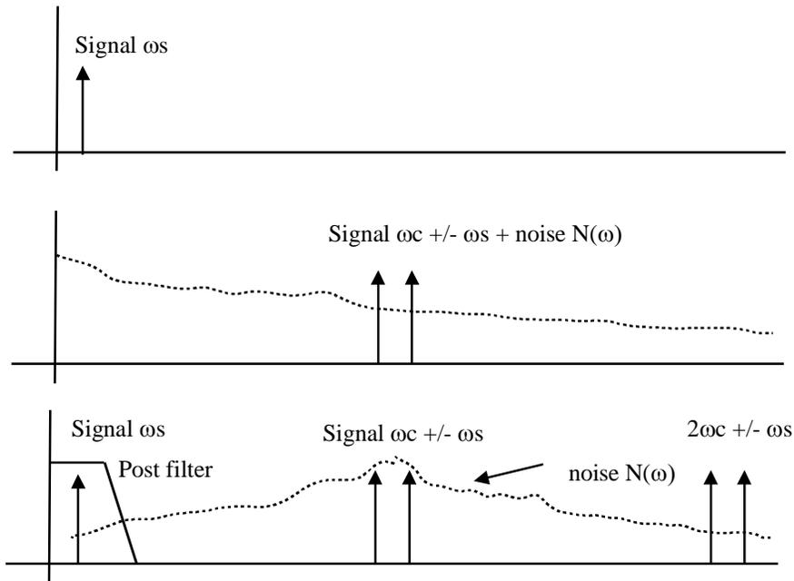
**Fig 4: a) Scan signal b) Received modulated signal plus noise c) Detected Signal**
