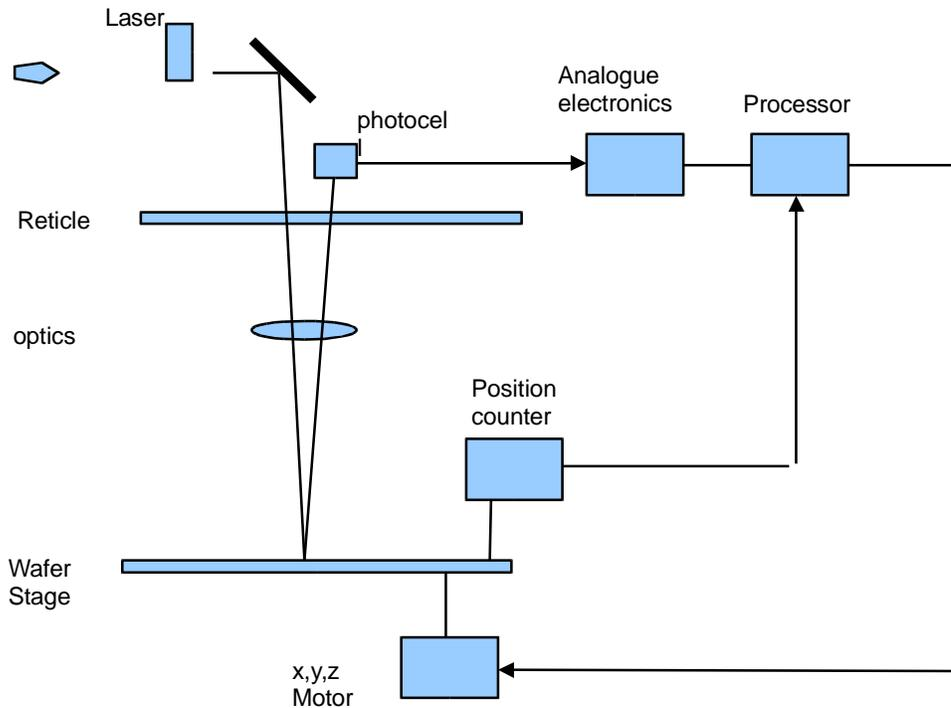
**Fig 2 Alignment System**
